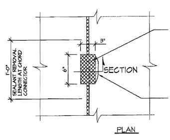
SEALANT POCKET AT CHORD CONNECTOR ANGLES. REMOVE SEALANT AND ADJACENT CONCRETE SPALLS, WIRE WHEEL EXPOSED STEEL TO NEAR WHITE CONDITION, INSPECT WELDS, REPORT BROKEN WELDS TO ENGINEER PLACE NEW SEALANT IN AREA OF REMOVED SEALANT AND FRACTURED CONCRETE
