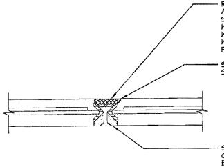
REMOVE SEALANT AND SPALLED CONCRETE AT CHORD CONNECTOR. CLEAN EXPOSED STEEL TO NEAR WHITE CONDITION WITH WIRE WHEEL, INSPECT WELDS AND COAT METAL WITH ZING RICH PRIMER. REPORT BROKEN WELDS TO ENGINEER BEFORE RESEALING. PLACE SEALANT IN REMOVAL AREA
