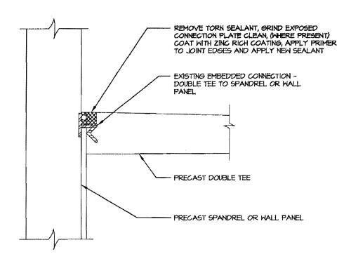
NOTE: STEEL CONNECTIONS WILL NOT BE PRESENT AT ALL LOCATIONS. AT LOCATIONS AWAY FROM CONNECTORS, REMOVE SEALANT, CLEAN EDGES, PRIME AND SEAL.
