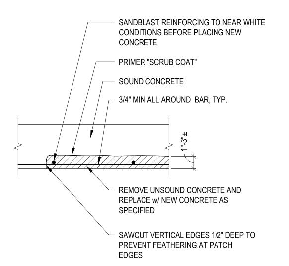
UNDERSIDE SLAB RESTORATION 1" = 1'-0" @ 22"x34" SHEET
