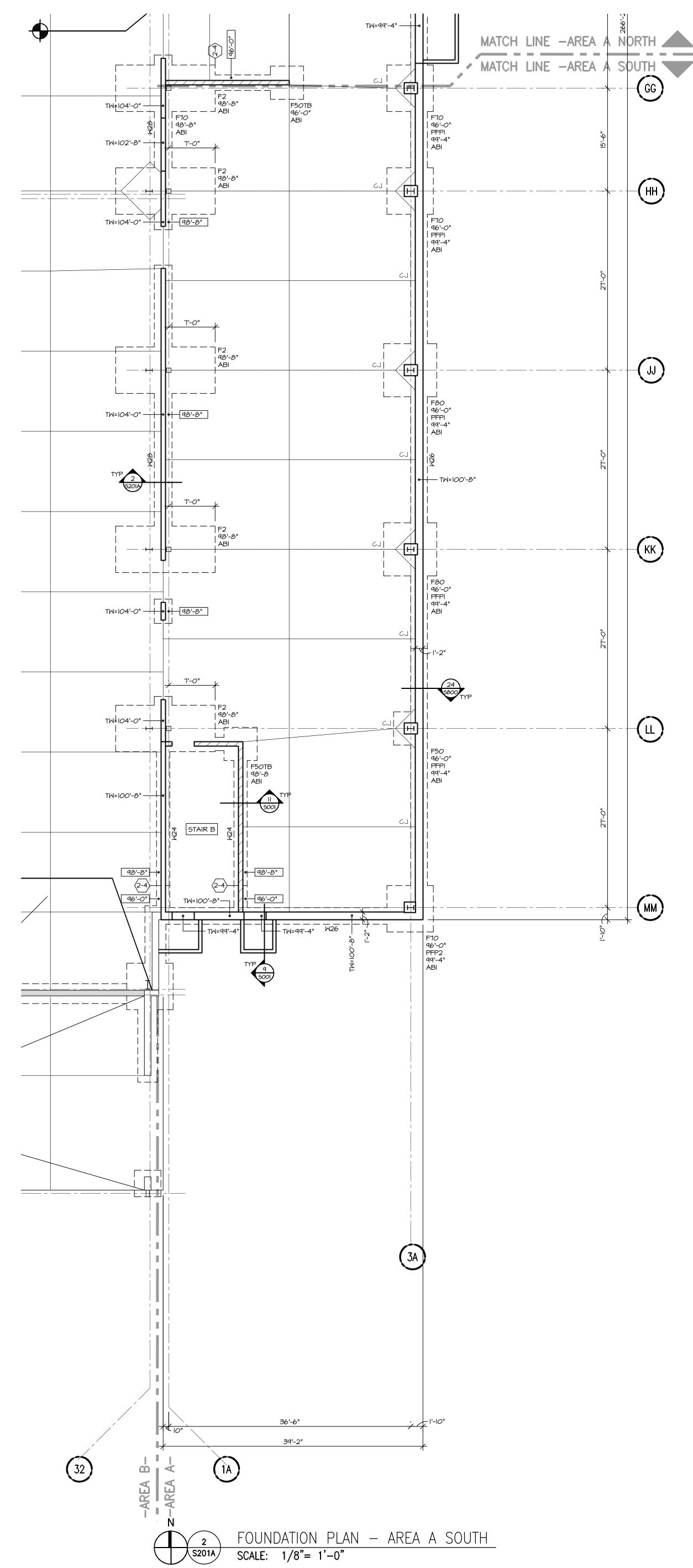
1) FINISH SLAB ELEVATION = 100'-0", TYP UNO
