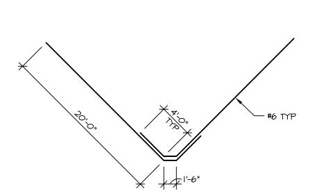
3 PAVILION SLAB REINFORCEMENT 5201B SCALE: NONE
