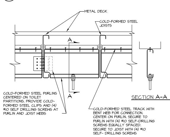
5 COLD-FORMED STEEL FRAMING **5211B** SCALE: 3/4"=1'-0
