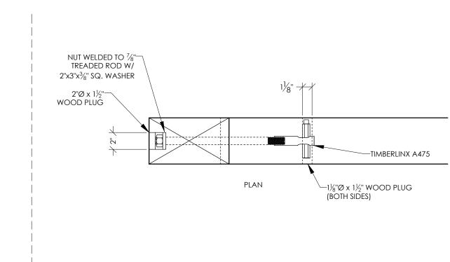
3 TYPICAL HIDDEN BOLT DETAIL SCALE: NONE
