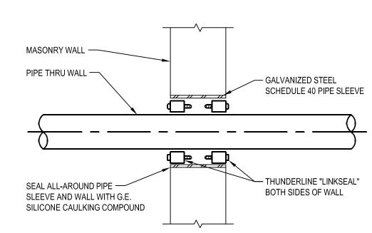
PIPE THROUGH EXTERIOR BELOW GRADE WALL DETAIL M801 SCALE: NONE
