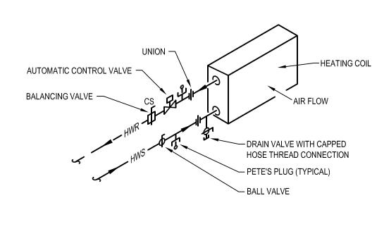
TYPICAL PIPING TO HOT WATER BOOSTER COIL DETAIL √ M801 / SCALE: NONE
