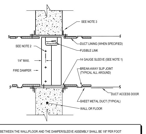
1. CLEARANCE BETWEEN THE WALL/FLOOR AND THE DAMPER/SLEEVE ASSEMBLY SHALL BE 1/8" PER FOOT OF WIDTH AND HEIGHT. MINIMUM CLEARANCES SHALL BE 1/4" FOR ANY SIZE DAMPER/SLEEVE ASSEMBLY. THE MAXIMUM OPENING SHALL NOT EXCEED 1/8" PER FOOT PLUS 1". MOUNTING ANGLES SHALL OVERLAP WALL BY 1" MINIMUM ON ALL SIDES.
