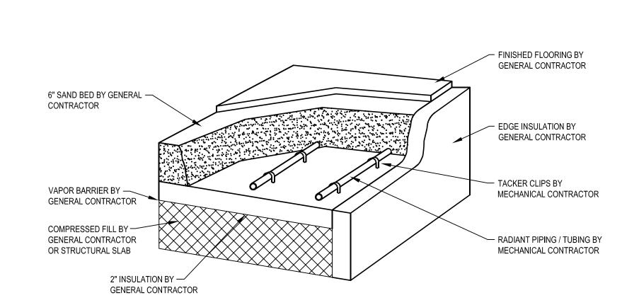
HYDRONIC IN - FLOOR HEATING DETAIL M801 SCALE: NONE
