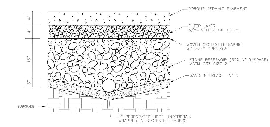
POROUS ASPHALT PAVEMENT SECTION
