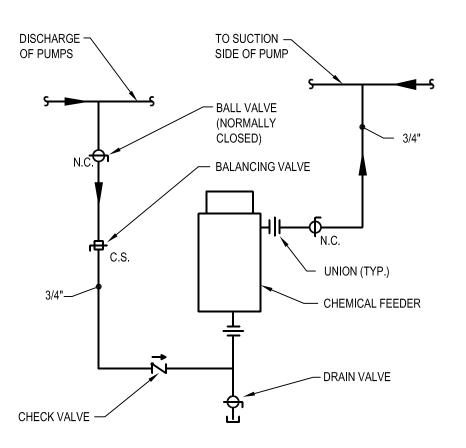
CHEMICAL FEEDER PIPING DETAIL M801 SCALE: NONE
