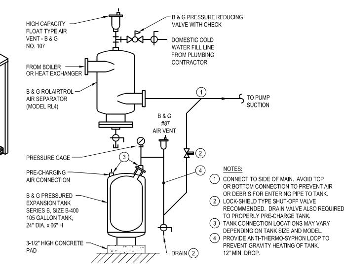
VERTICAL EXPANSION TANK WITH AIR SEPARATOR DETAIL √ M801 SCALE: NONE
