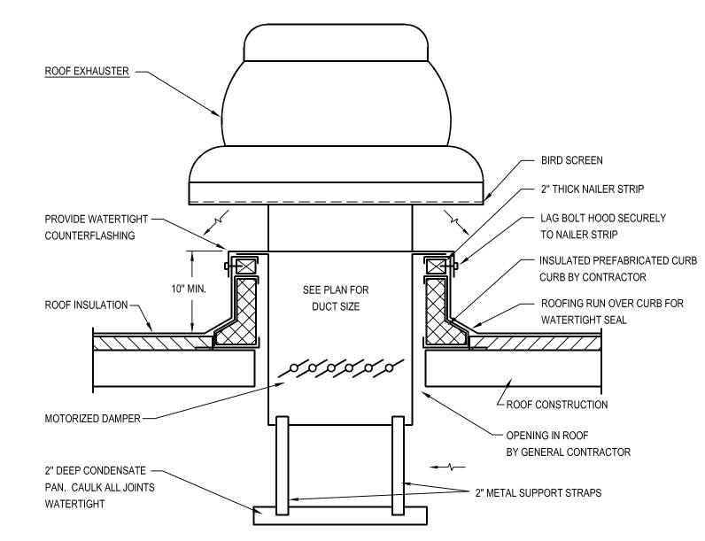
TYPICAL ROOF EXHAUSTER DETAIL WITH CONDENSATE PAN √ M801 / SCALE: NONE
