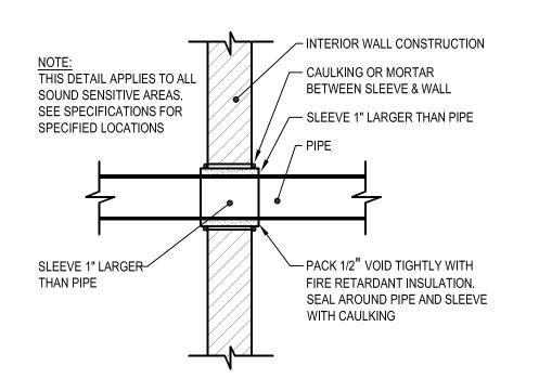
PIPES THROUGH WALLS DETAIL \ M801 / SCALE: NONE
