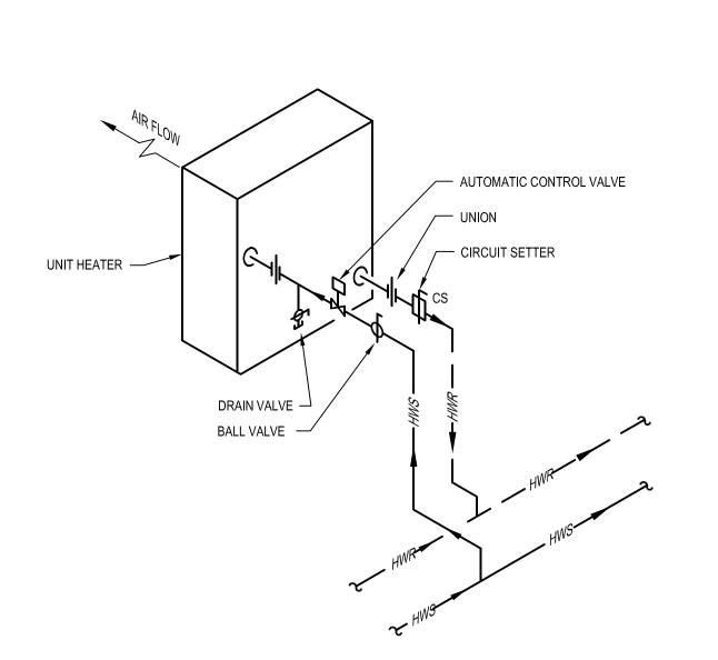
HOT WATER UNIT HEATER PIPING DETAIL M801 SCALE: NONE
