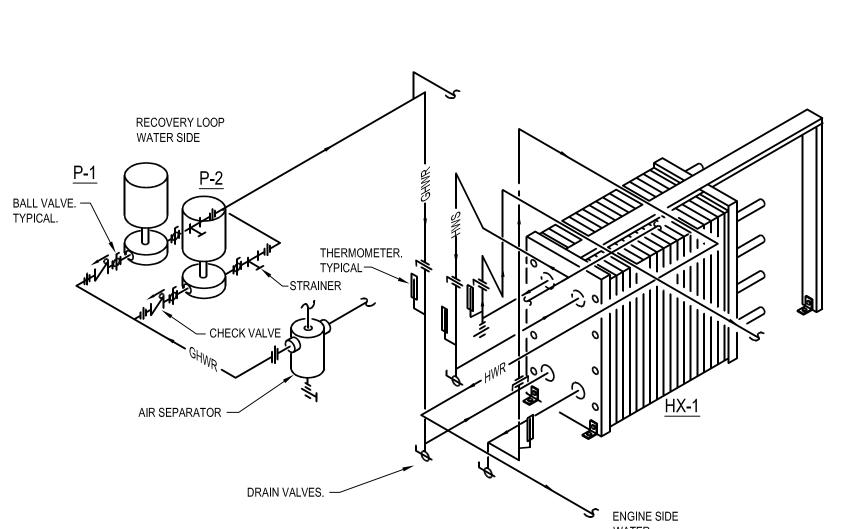
PLATE AND FRAME TYPE HEAT EXCHANGER PIPING DETAIL M801 SCALE: NONE
