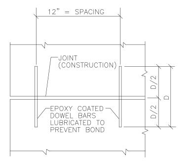
PAVEMENT DOWEL LENGTH THICKNESS | DIAMETER 1-1/4" 16" 1-1/2" 18"
