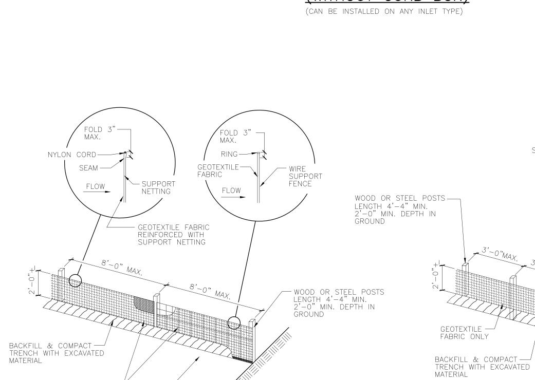
NOTE: ADDITIONAL POST DEPTH OR TIE BACKS MAY BE REQUIRED IN UNSTABLE SOILS ALTERNATE "A"
