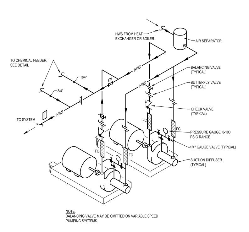
DUPLEX BASE MOUNTED HOT WATER PUMP PIPING DETAIL √ M801 SCALE: NONE
