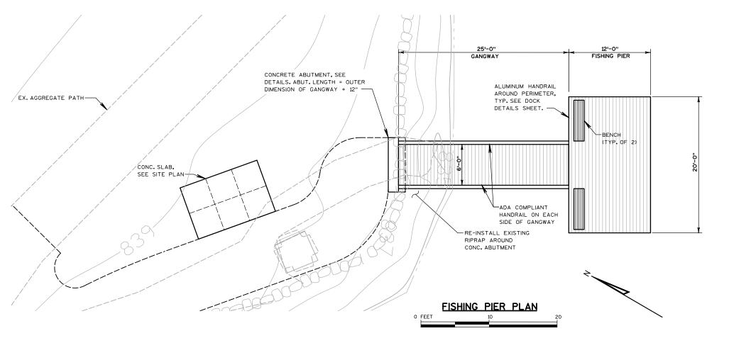
PIER MANUFACTURER IS RESPONSIBLE FOR DESIGN OF THE FLOATING PIER SYSTEM AND COORDINATION WITH THE GENERAL CONTRACTOR TO PROVIDE A COMPLETE SYSTEM WHICH IS FUNCTIONAL THROUGHOUT THE DESIGN WATER LEVEL RANGE.
