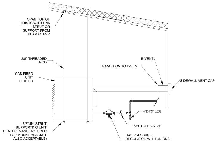
2 GAS FIRED UNIT HEATER M100 SCALE: NO SCALE
