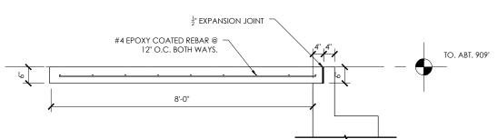
5 NORTH RETAINING WALL SECTION VIEW SCALE: 1" = 1'-0"
