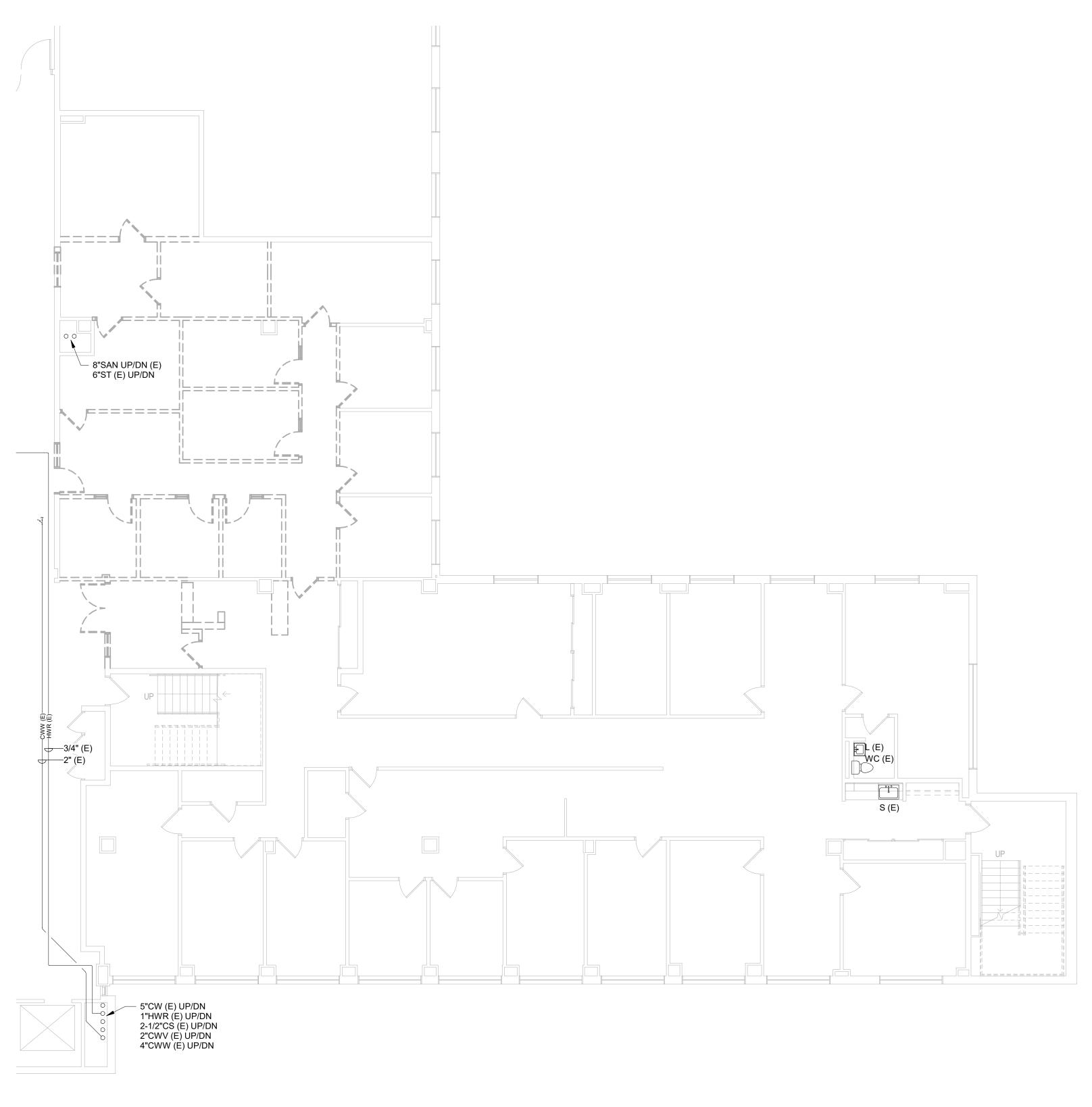
**DEMOLITION PLAN - SOUTH - PLUMBING** ໌ 1 ີ P1.0 SCALE: 1/8" = 1'-0"
