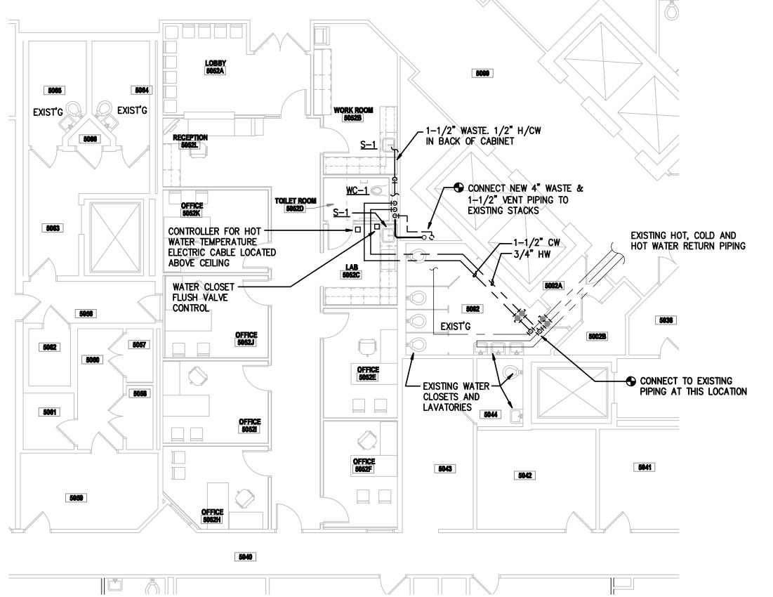
PARTIAL FLOOR PLAN - PLUMBING NEW WORK
