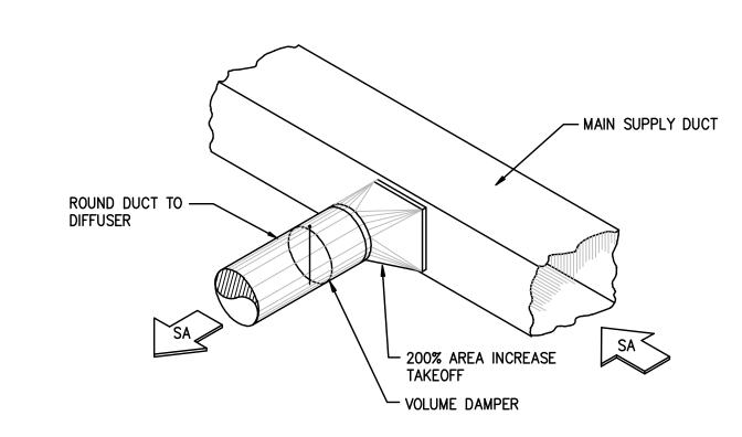
BRANCH DUCT TAKEOFF DETAIL NOT TO SCALE
